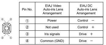
\* Maximum cable length for operation of the WAT-600CX depends on which lens is used. For example, 100m is the maximum cable length for the WAT-600CX when an auto-iris lens with a current consumption of 50mA is applied.
