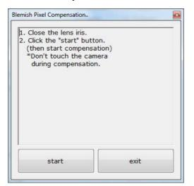
Fig. 18 Blemish Pixel Adjustment window
